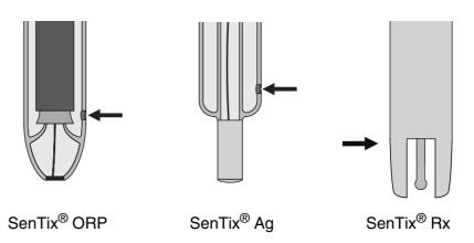
SenTix<sup>®</sup> ORP, SenTix<sup>®</sup> Ag and SenTix<sup>®</sup> Rx: The level of the reference electrolyte must be at least 2 cm above the level of the solution.
